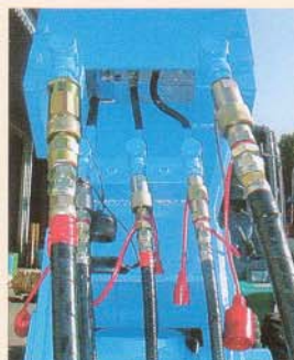
Swivel joints and quick-and-easy couplers
