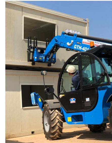
14m/18m Boom 4t Payload
